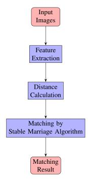
Figure 3. Process-flow of the proposed matching algorithm.
