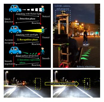
Fig. 1. Proposed visual interaction and robotic platform (upper left: three phases, upper right: robotic wheelchair with sensors and a projector, bottom: local light projection on a pedestrian in the real-world experiment).
