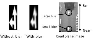
Figure 7: Example of optical blur.
