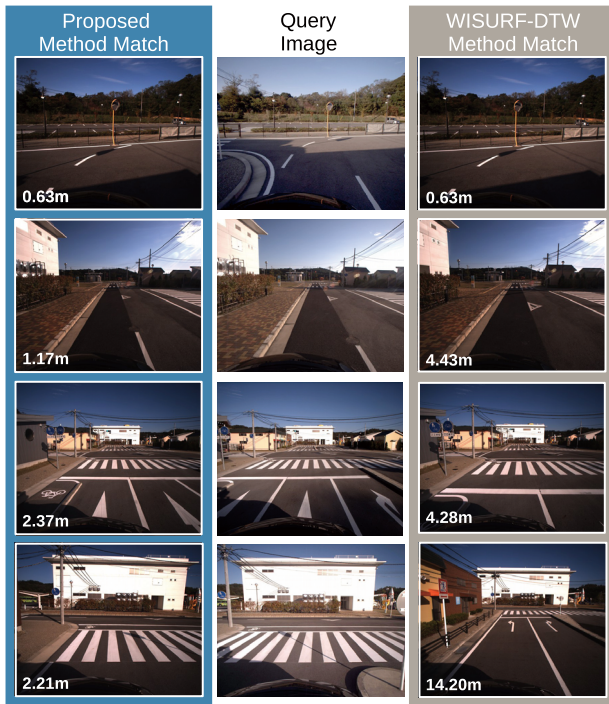
Fig. 5 Example image matching results. The top two rows show image matching in the same lane, whereas the lower two show matching where the query lane is different from the database lane. Current localization errors are shown in the bottom left-hand corner.
