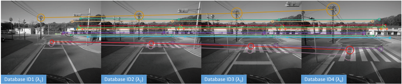
Fig. 7 Sample “feature scale tracklets”, with each tracklet shown in a different color. The circles represent the feature positions and their diameters show the feature scale, illustrating the scale increase along the tracklet. Only some of the tracklets are shown for clarity.
