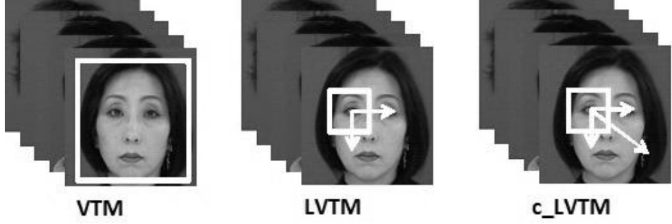
Fig 4 The difference of VTM, LVTM and the proposed c-LVTM. VTM learns a global linear mapping on the whole face image plane; LVTM learns location specific linear mapping for each local patch; c-LVTM learns linear mappings that are both location specific and local 3D structure specific.
