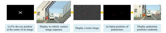
Figure 4. The procedure to evaluate the detectability by a human subject. (s) indicates the subject's action.
